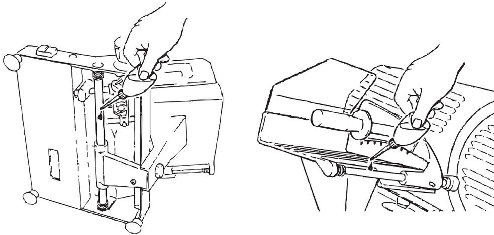
After a given period of service an unusual noise may occur because of the belt bedding. In this case, tighten the belt-stretcher on the side of the motor under the machine base.
